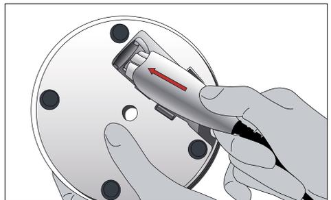
Connect the power cord with the power supply and the power pack. Make sure that the power cord is easily accessible at all times and can easily be disconnected from the power supply. The Power On indicator on the power pack lights up in green and the illuminated ring on the charging base briefly lights up in blue.
