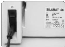
1. To switch off the apparatus, remove the power cord from the socket of the apparatus or the mains socket.
