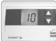
6. Selecting the mixing time: The mixing time can be set between 1 and 30 seconds. In general a mixing time of 10 seconds can be used (unless other mixing times are recommended by the material supplier in the instructions for use). By default, the Silamat S6 was set to 10 seconds. The last used mixing time remains stored even if the apparatus had been switched off in the meantime.
