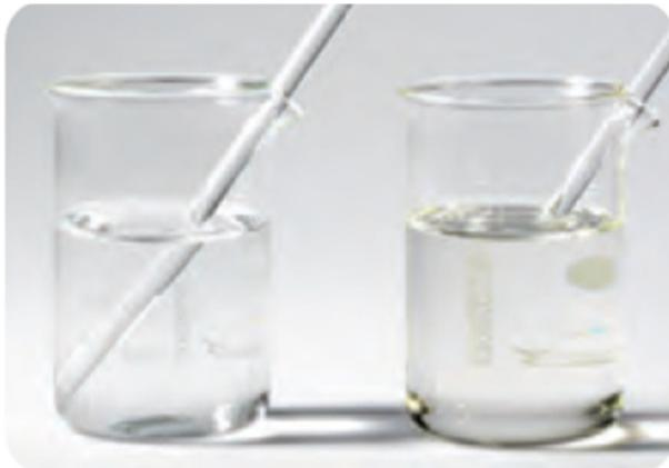
Fig. 5: Illustration of refractive index with glass rods in water (left) and monomer mixture with coordinated refractive index (right)
