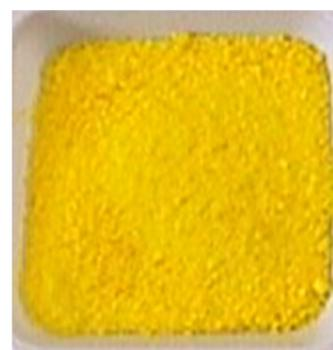
Fig. 12a-c: Light initiators contained in Tetric EvoCeram Bulk Fill in their pure form:
