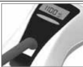
Position the light probe directly on the centring gauge and flush on the sensor surface.
