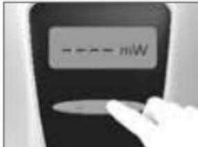
Press the (+) button until the milliwatt program is selected and << ----mW >> is shown in the display.
