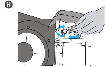
**H** Insert the heater plug into the intended connector. Secure the heater plug by rotating it 45°.
