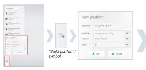
New investment ring or wax tree platform Click on the "build platform" symbol to create the wax tree and go to the selection menu for the required settings. *Machine:* determines the ring base size 100 g or 200 g *Material:* determines the final IPS e.max<sup>®</sup> Press material *Shade:* final tooth shade
