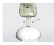
Adjusting the press channel width The width of the press channel can be selected between 2.5 mm and 3.0 mm.
