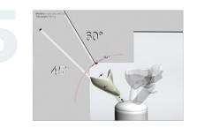
Adapt angle The angle of the individual press objects can be individually adjusted within the Sprue Guide.
