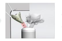
Adjusting the press channel length and position The length of the press channel and its position on the press object and wax tree base can be individually adjusted.
