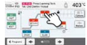
When the furnace is delivered ex factory, Ivoclar Vivadent programs are write-protected. The write-protection can be deactivated in the Options menu, where additional program options are available.
