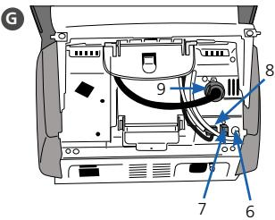
H Insert the heater plug into the intended connector. Secure the heater plug by rotating it 45°.
