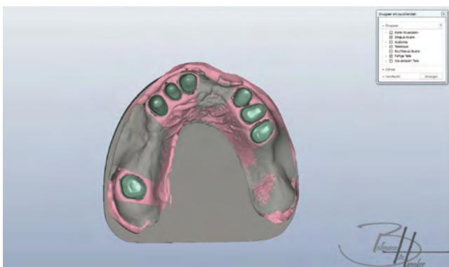
**Fig. 5** As gingiva components can be shown in the software, the shoulder height of the telescopes could be determined precisely.
