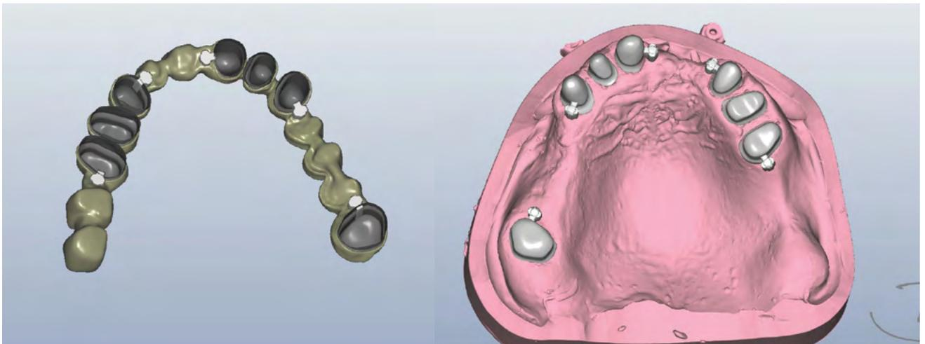
**Figs 9 and 10** In order to allow for possible loss of friction during the construction of the framework, small spacers for friction attachments were added to the primary telescopes. The virtual attachment parts were loaded into the design software as so-called mash-ups for visualization from the database. Mash-ups are applications which cannot be provided by the actual software, however, they can be added.
