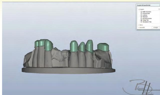
**Fig. 4** The primary path of insertion of the model was defined in the CAD software according to the shaft of a bur which was placed in the parallelometer. In this way, the situation corresponded exactly to the insertion direction defined in the parallelometer.
