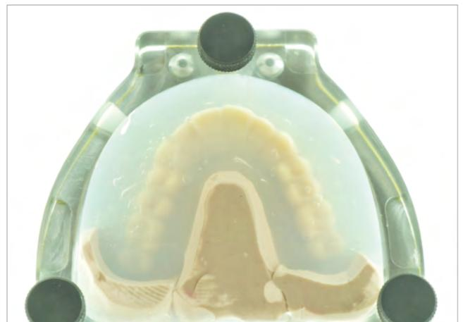
**Fig. 13** The clear silicone Transil F has a Shore hardness of 72. The screws are released after a short setting time of 12 to 15 minutes and the two flask halves are separated.
