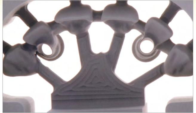
**Fig. 13b** Pre-sintered metal framework for the fabrication of the final restoration
