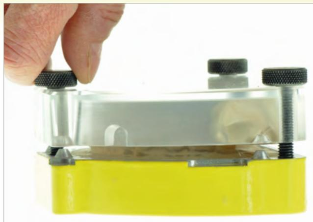
**Figs 19 and 20** The flask is closed by placing the top half onto the bottom half. When a perceptible resistance is felt, the three screws are inserted and slowly and carefully tightened one by one, giving each screw one to two turns.
