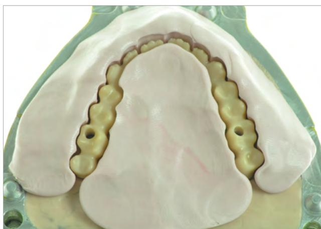
**Fig. 16** Before the composite resin was pressed on the zirconium oxide framework, all the dimensions were checked against the previously fabricated silicone matrix. At this stage, the framework could still have been adjusted if necessary.
