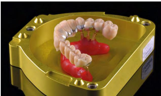
**Fig. 13** ... transferred to the framework using a silicone template and wax injector. The gingival areas were removed. The modified framework was placed with a holder on the lower half of the flask.
