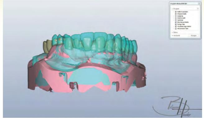
**Fig. 8** The secondary crowns were designed according to the usual requirements, however in a virtual construction. The hardness of milled NP alloys is lower than that of cast NP cast alloys, which means a stronger framework must be designed.
