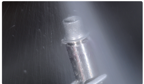
Optional: Cleaning with an instrument and a steam cleaner. It is important to remove all the wax meticulously.
