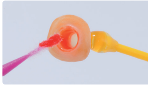
Etching with IPS Ceramic Etching Gel for 20 s and subsequently rinsing it off with water.
