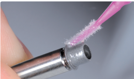
Monobond Plus is applied to the clean bonding surface and allowed to react for 60 s. After the reaction time, any remaining residue is dried with blown air that is free of water and oil.
