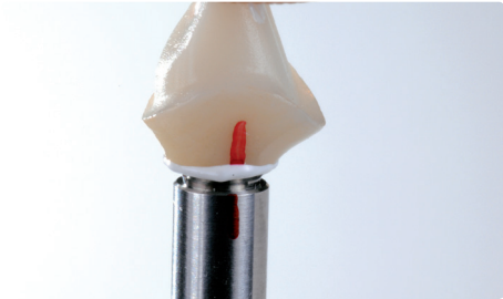
The ceramic structure is placed on the base in such a way that the position markings are aligned.
