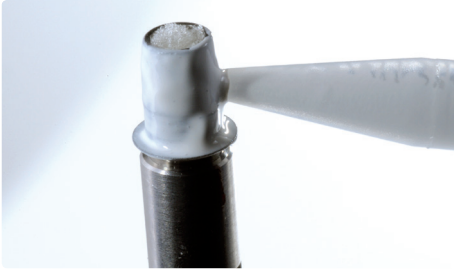
A thin layer of Multilink Hybrid Abutment is directly applied from the mixing syringe to the bonding surface of the base.
