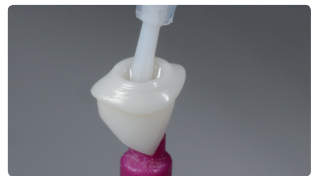
Monobond Plus is allowed to react for 60 s and then dried with blown air.
