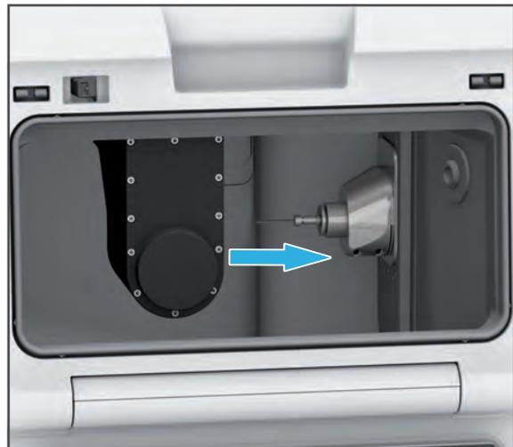
7. Clean the left side of the milling arm (B axis, pos. (3))
