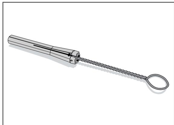
7. Take a small amount of the collet chuck grease from the spindle service set and apply it to the collet flanks (1).
