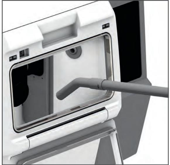
3. Clean the viewing window (1) and the seal of the front flap (2) with a soft cloth, dampened with tap water and a mild, pH neutral detergent.
