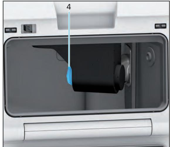
9. Swivel the milling arm to the starting position (B axis)
