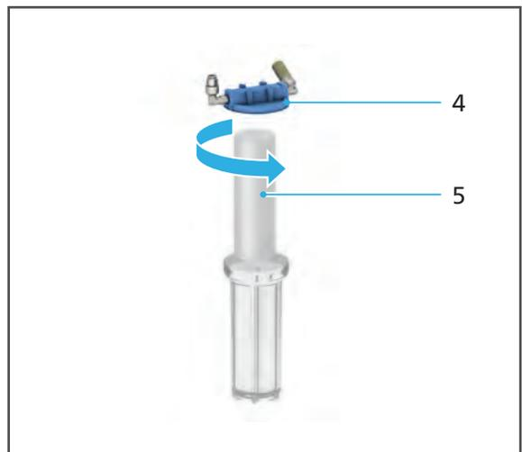
6. Rinse the filter container with fresh water, collect the water and dispose of according to the specifications (Safety Data Sheet PrograMill Fluid).
