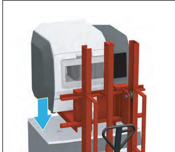
5. **When using the PrograMill Base cabinet:** Position the device above the cabinet so that the feet (1) can be placed in the recesses (2) provided on the cabinet.
