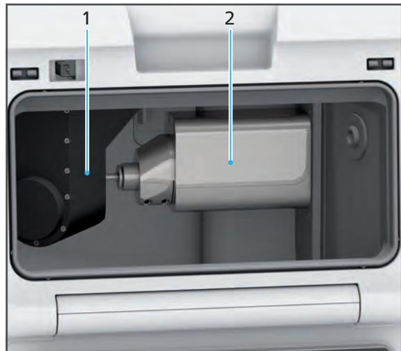
6. Swivel the milling arm (B axis)
