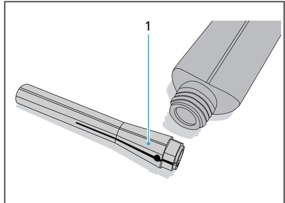
8. Screw the collet into the spindle until it stops using the screw-in piece.
