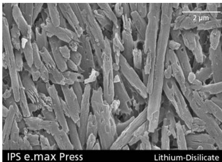
Fig. 3: Microstructure of IPS e.max Press (SEM, etched with HF vapour for 30 s)
